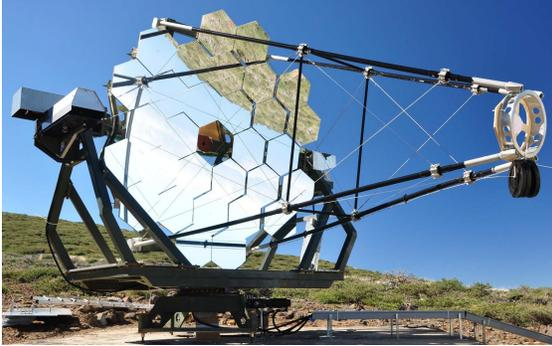
Figure 1: The FACT telescope at La Palma with the newly refurbished mirrors awaiting the camera to be installed.
