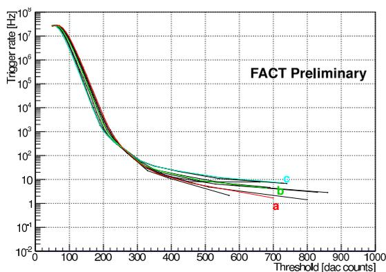
**Figure 6:** FACT rate scans of one night indicating variable atmospheric conditions. The scans marked a,b and c correspond to the sky images in figure 7.
