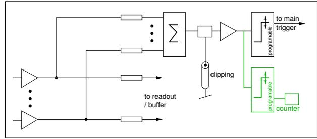
**Figure 9:** Using two independent comparators, rate scans can be done during data-taking.
