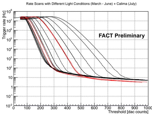
**Figure 5:** FACT rate scans same as figure 4, including additional four nights with Calima marked in red.
