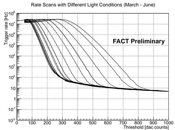
**Figure 4:** FACT rate scans for similar zenith and good weather conditions. The leftmost line corresponds to dark nights and the rightmost is from  $\sim 90\%$  fullmoon.
