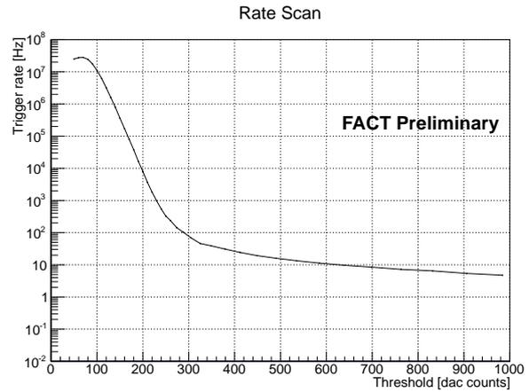
**Figure 3:** FACT rate scan. While for low thresholds the rates are dominated by accidental triggers, for high thresholds the dominant contribution is from cosmic ray particles (mainly hadrons). The counters saturate at  $\sim 10^7\text{ Hz}$ .
