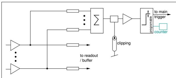
**Figure 8:** Schematics of the trigger system used in FACT.
